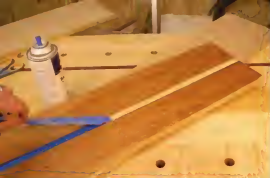
Peel away problems. A strip of blue tape protects the inside of the groove from finish materials and keeps the fit tight.
